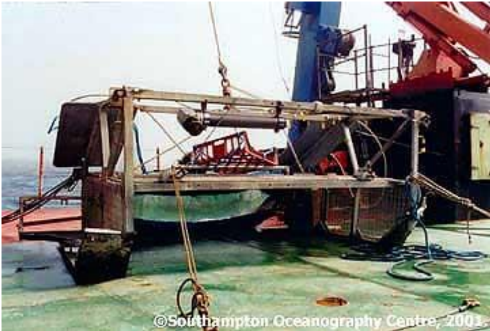
Picture 3.4: Epibenthic Sledge on the deck of a research vessel. (Southampton Oceanographic Centre)
