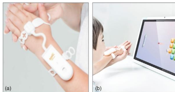
Figure 18: Component of the virtual reality device developed for upper-limb rehabilitation in children with disabilities. (a) Band-like wrist attachment device with two inertial measurement unit sensors on the hand dorsum and distal forearm. (b) Software in combination with a personal computer and a screen [123]
