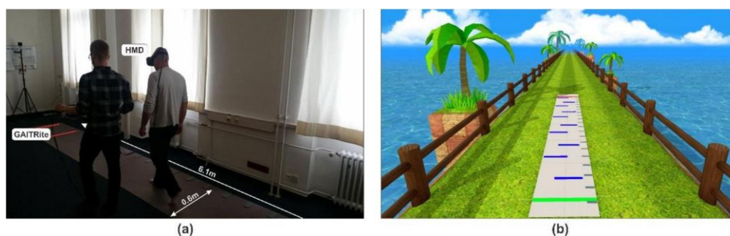
Figure 14: Experimental setup: (a) A participant walks in the real workspace with a head-mounted display (HMD) over the GAITrite ® walking surface. (b) Participant's view of the virtual environment on the HMD. [249]
