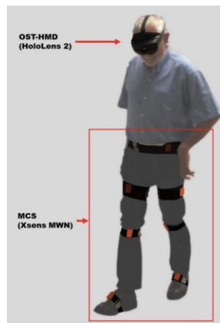
Figure 16: Patient who has had a stroke wearing the ARISE system, including the optical see-through head-mounted display (HoloLens 2) and the sensor-based motion capture system (Xsens MVN) [252]
