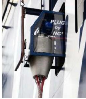
Figure 12. Connecting the ship to the ground network using an automated procedure.
