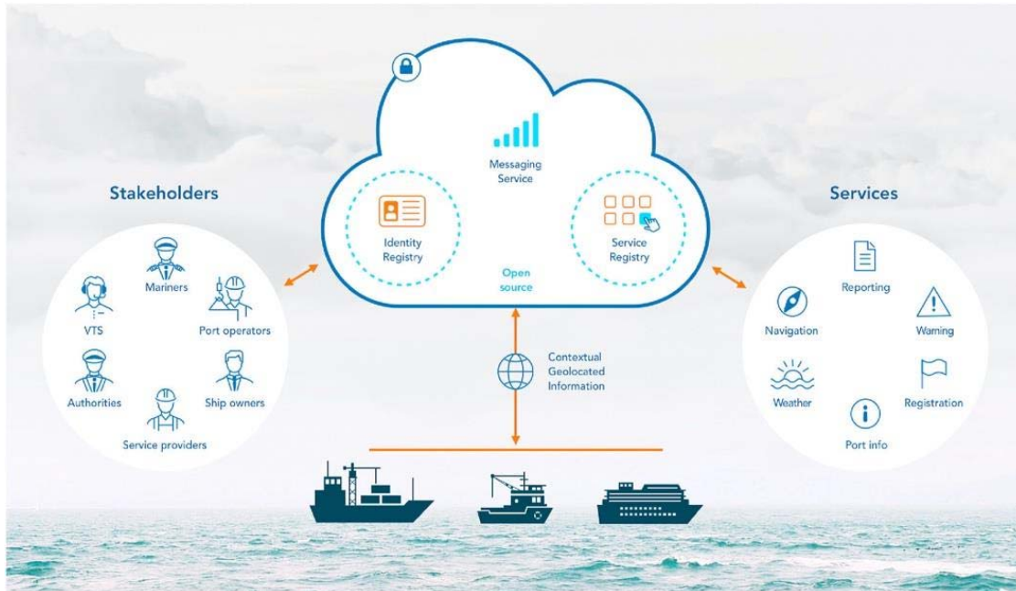
Diagram No.2 - Diagram of the operation of the MCP platform (Zhang et al, 2021)
