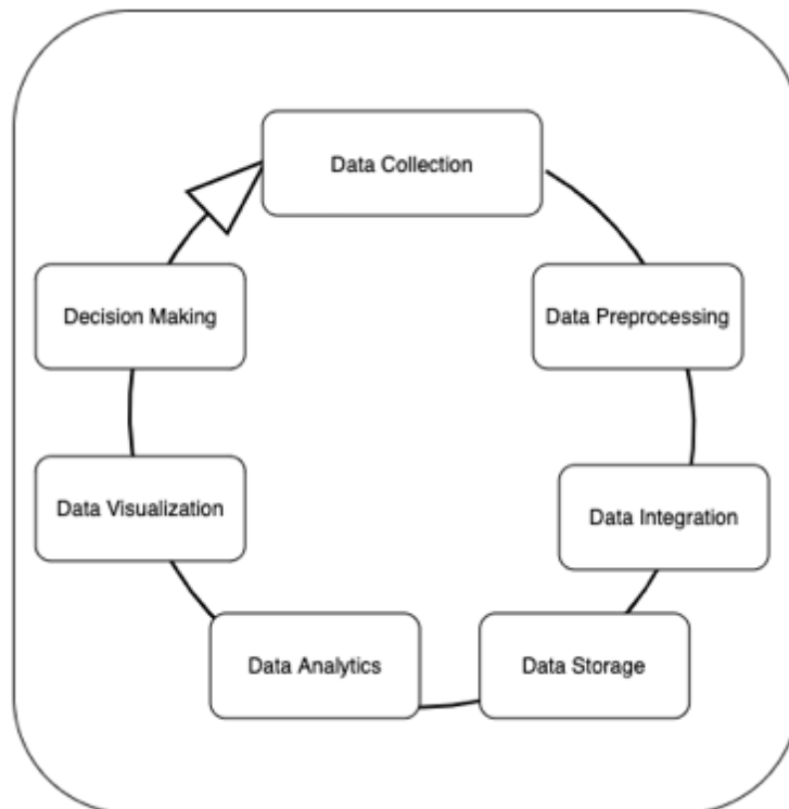
Figure 4: Data management flow in smart grid.
