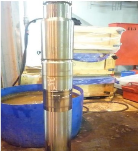
Photo 3.3: Exhaust valve shaft for grinding [1]
