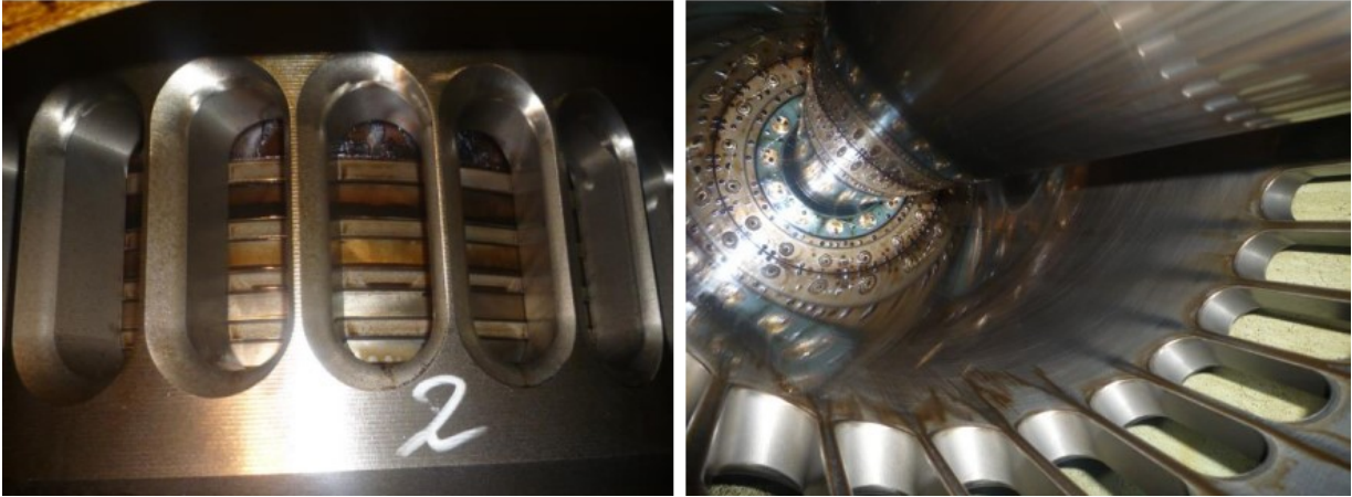
Photo 3.7: Checking the rings and liners of the second cylinder on the engine after 250 hours of operation. A small amount of carbon is observed inside the upper part of the rings [1]
