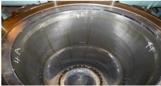
Photo 3.5: Check of the surfaces of the cylindrical sleeve with ID 4 [1]
