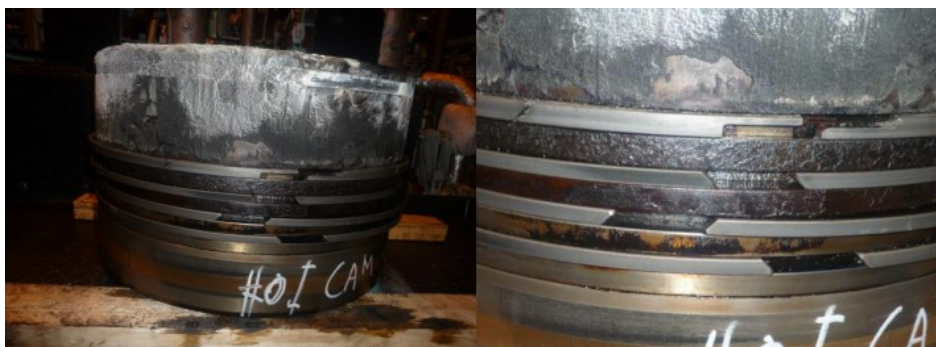
Figure 3.7: Check piston with ID 1 on top and in its grooves [1]
