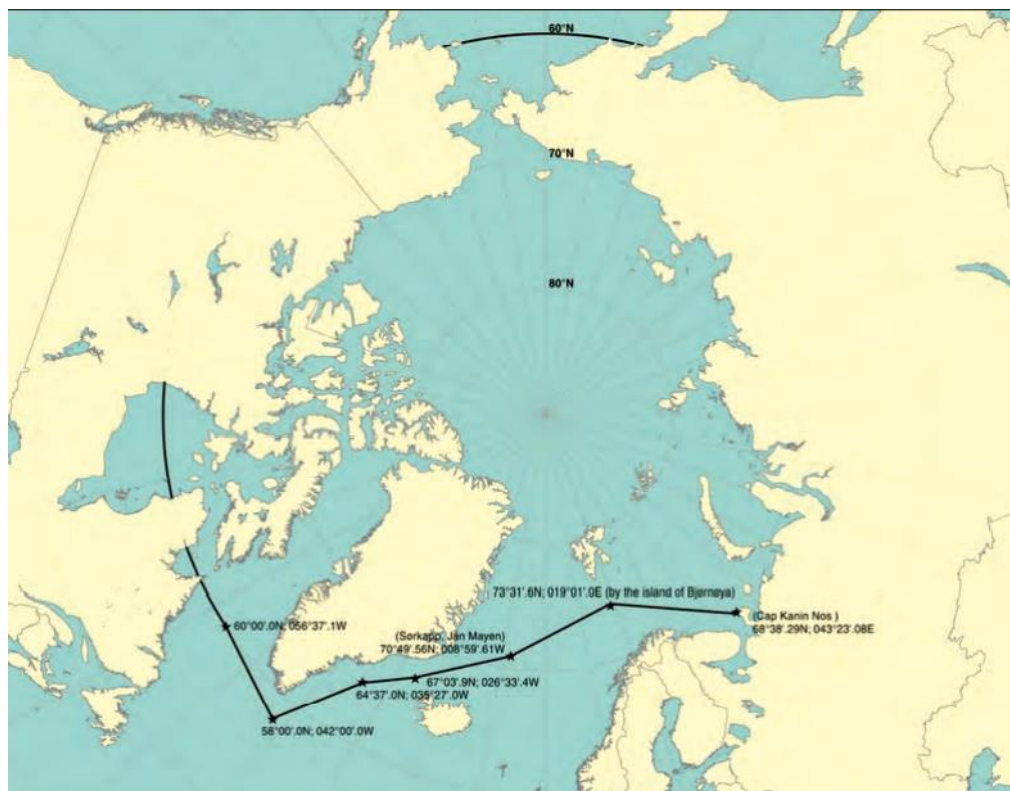
Figure 3: Maximum geographical extent of the Polar Code's area of application in the Arctic (International Maritime Organization, IMO, 2017)
