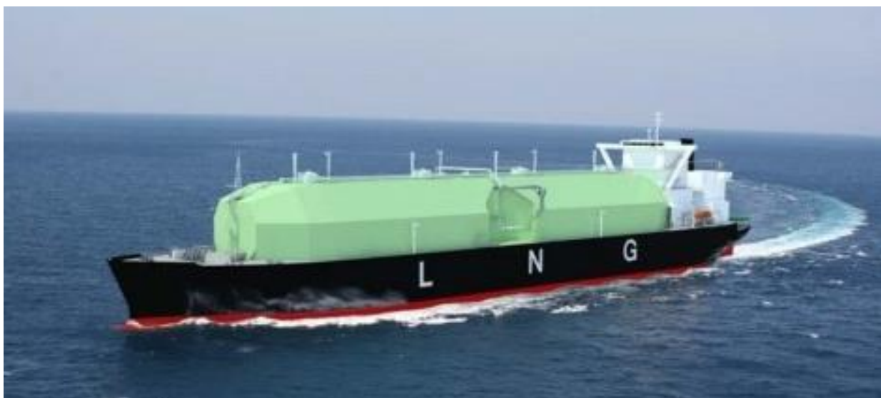
Εικόνα 37. Sayaringo. Πηγή: SAYARINGO STaGE- Next Generation MOSS-type LNG Carrier with hybrid propulsion plant - Mitsubishi Heavy Industries Technical Review Vol.53 No.2(2016) (mhi.co.jp)
