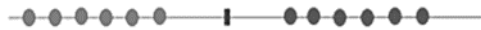
Figure 7. A 1-dimensional linearly separable set of data. The data can be easily separated in two classes by choosing an appropriate point on the x-axis.
