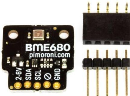
The sensor communicates with a microcontroller using I2C or SPI communication protocols. The gas sensor can detect a broad range of gases like volatile organic compounds (VOC). For this reason, the BME680 can be used in indoor air quality control.
