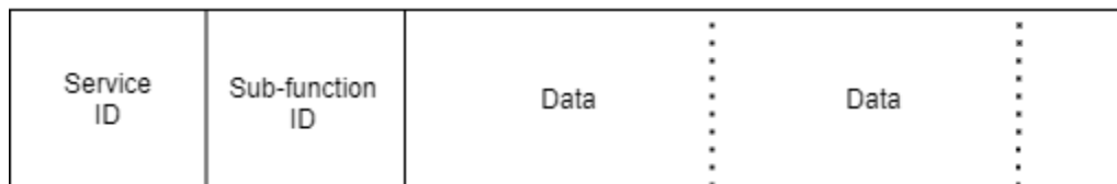
Figure 5. UDS request packet layout
