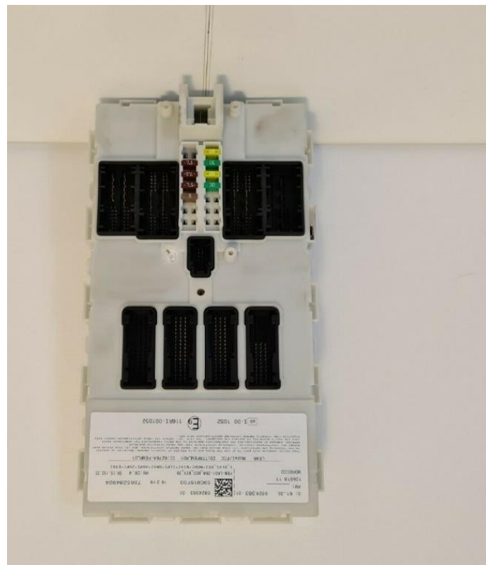
Figure 23. FEM ECU used in test bench
