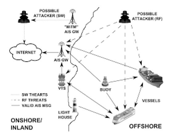
There are three (3) categories of identified threats which are related to the AIS, meaning Spoofing (sending of false information), hijacking and availability disruption; however, it is possible to avoid all the threats if the AIS data is compared to other sources (Balduzzi et al, 2014).
