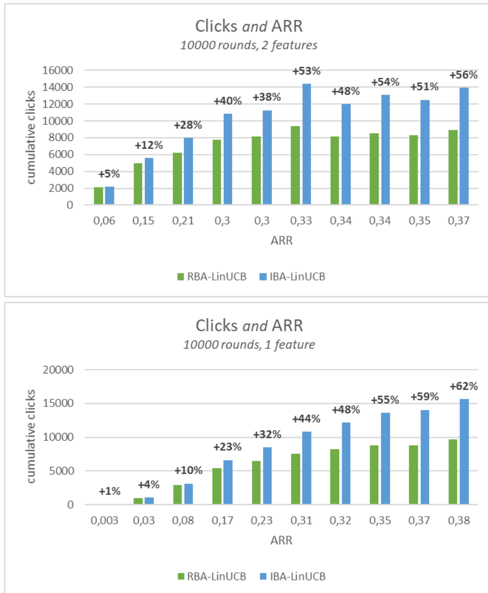
Figure 5.5. The accumulated clicks of RBA-LinUCB and IBA-LinUCB for d \in \{1, 2, 3\} , T=10000 , K=10 . The charts display the increase in IBA clicks as a percentage of the RBA clicks. The results were averaged over the 100 experimental repetitions for each dataset.
