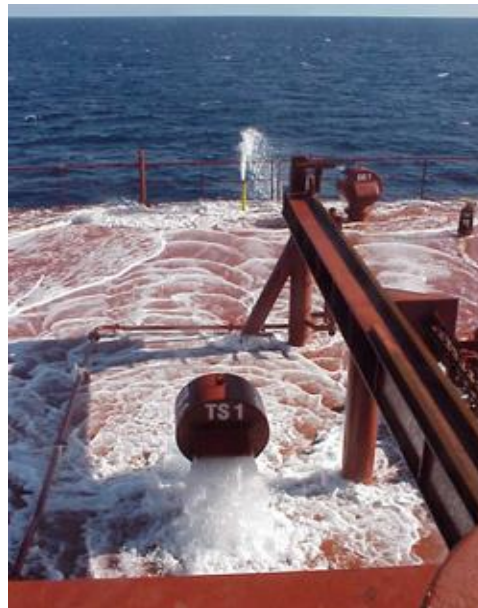
Εικόνα No.7: Ballast water is forced out an opening at the top of the ship in flow-through exchange
