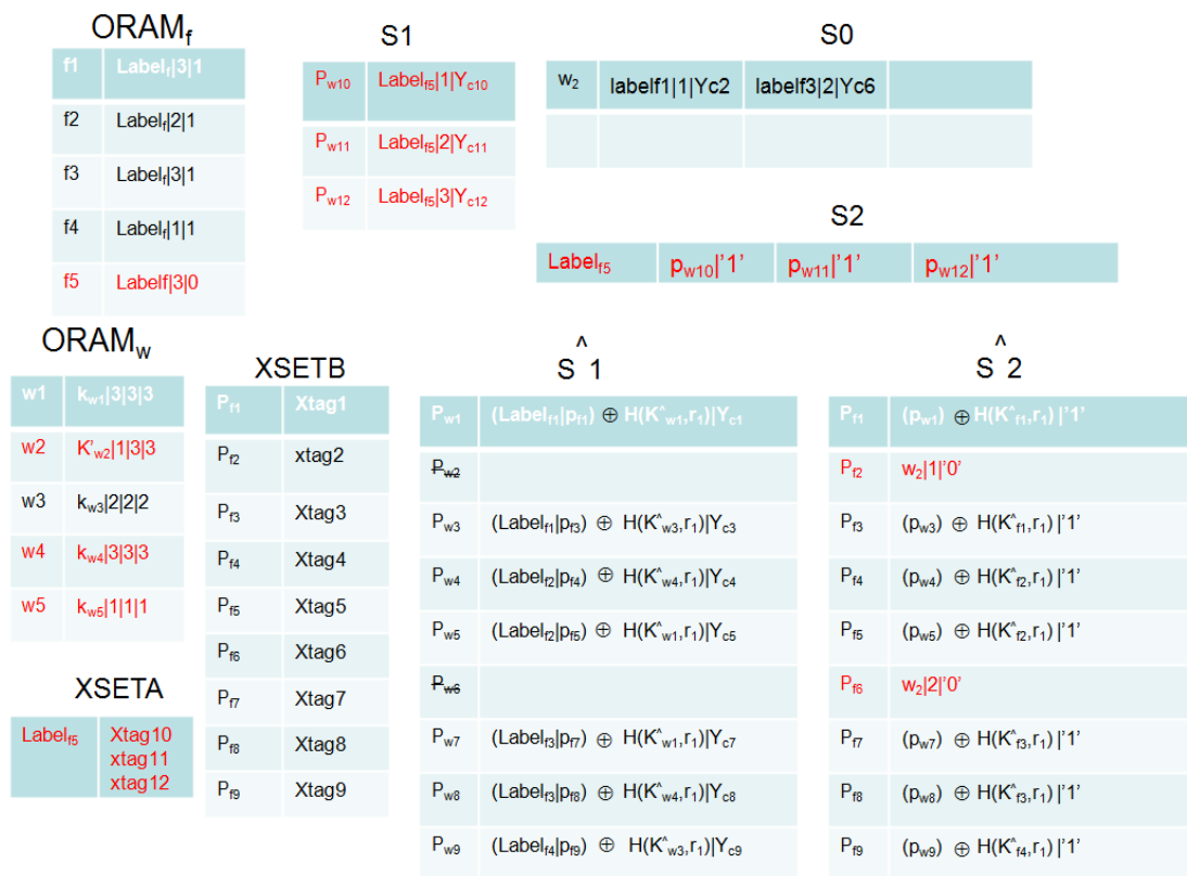
Figure 10.8 - State of structures after Add phase.
