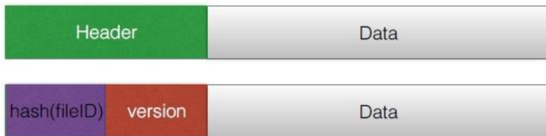
Figure 6.4 - Format of blocks that consist a file
