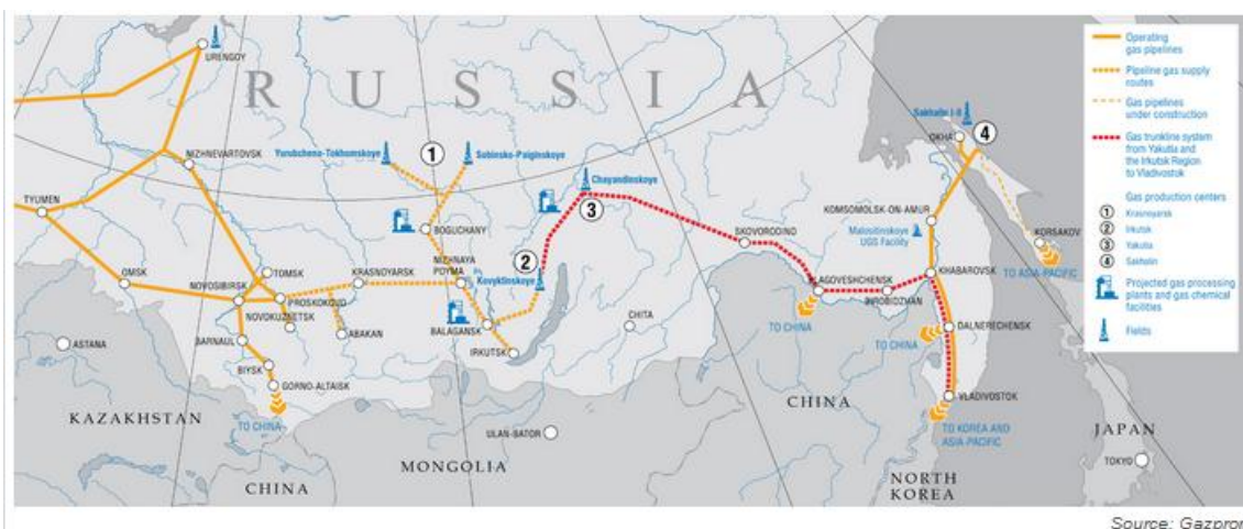
In late 2012, Gazprom announced plans to build a major trunkline (red line on map) from its interior gas fields to the Far East port city of Vladivostok. The pipeline could cost $13 million a mile. (Click to enlarge.)
