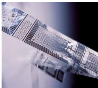
Flexible label with an aluminum antenna
