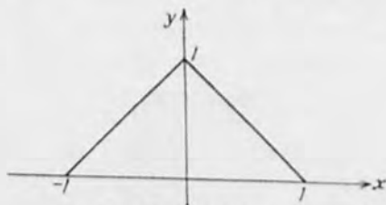
FIG. 10.—Graph of the function y = -x + 1, if x > 0; = x + 1, if x \leq 0.
