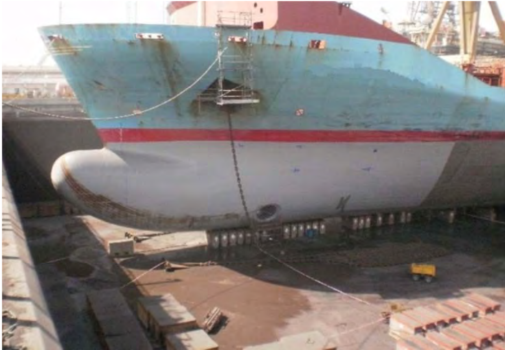
Picture 5: Container ship resting on keel blocks
