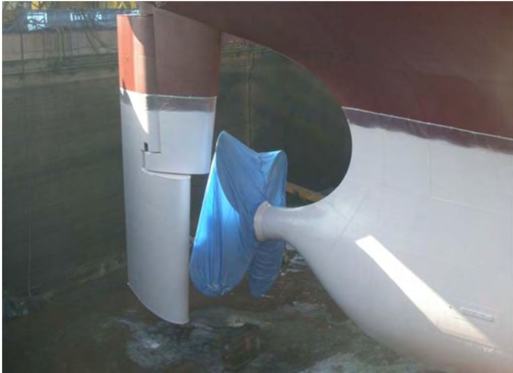
Picture 19: Protecting measures from silicon painting
