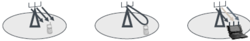
Figure 3 - Diversity Gain, Array Gain, Spatial Multiplexing[12]
