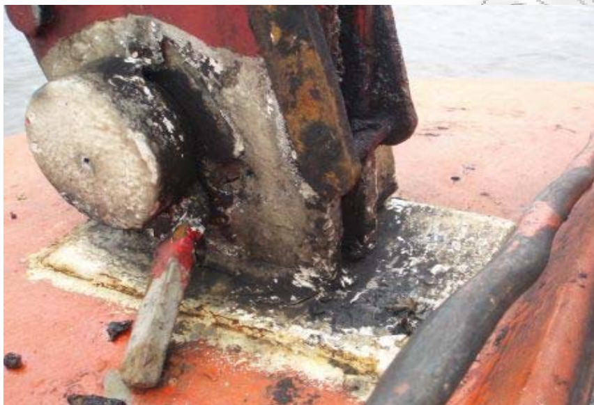
Εικόνα Γ1: Lifeboat release mechanism is defective
