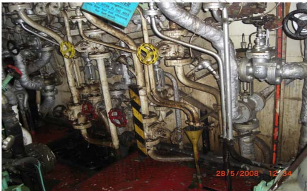
Εικόνες Γ7 & Γ8: The condition of the engine room is clearly hazardous, due to generalized oil dirtiness.
