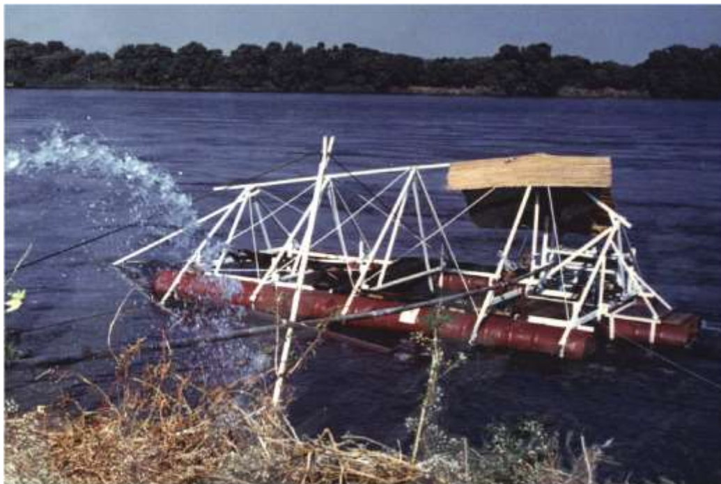
Figure 21 River current turbine on the Nile, Sudan, 1982 (source CNBC)
