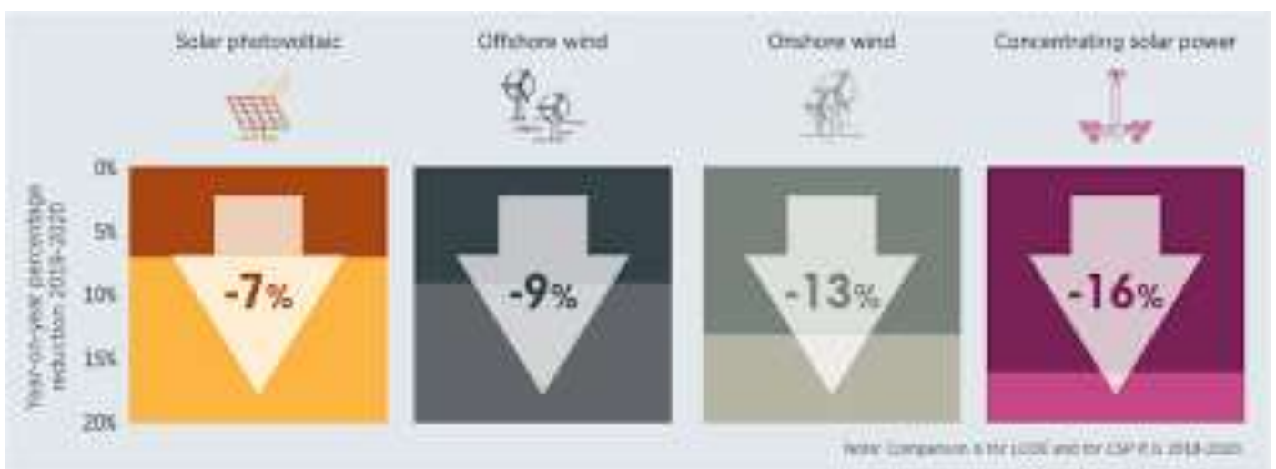
Figure 31 Global weighted-average LCOE from newly commissioned, utility-scale solar and wind power technologies, 2019-2020 (source IRENA)
