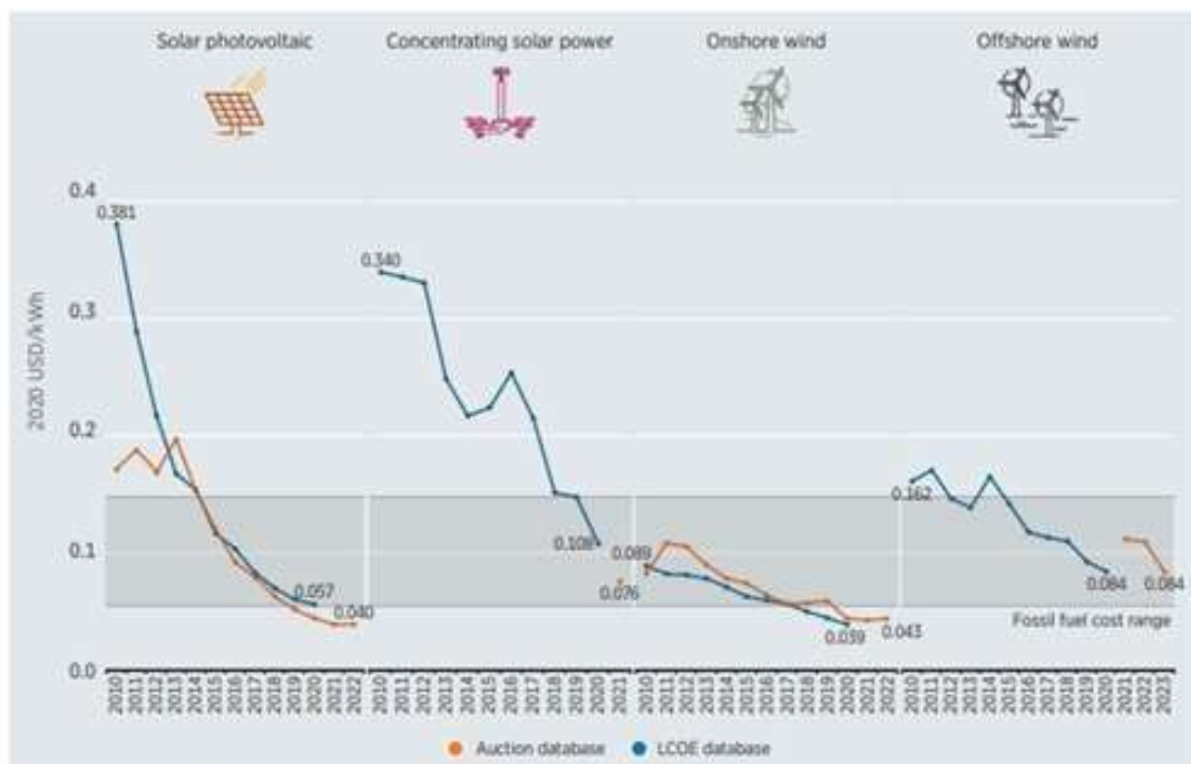
Figure 32 The global weighted-average LCOE and PPA/auction prices for solar PV, onshore wind, offshore wind, and CSP, 2010-2023 (source IRENA)
