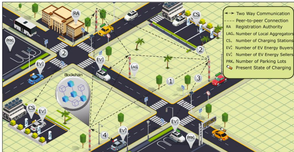
Figure 32. Proposed system model for energy trading. ① LAGs are interconnected in a P2P manner, all energy trading transactions are stored, audited and verified by the authorized LAGs. ② CSs send the energy trading request to the LAGs. They reply back with the notification. ③ Seller EV sends the energy selling request form PRKs to LAGs. ④ Buyer EV gets the information of nearest energy seller with distance and required time and expenses. Reprinted from “A consortium blockchain based energy trading scheme for Electric Vehicles in smart cities”, by Rabiya Khalid, Muhammad Waseem Malik, Turki Ali Alghamdi, Nadeem Javaid, Journal of Information Security and Applications , Volume 63, Article number 102998, December 2021. Copyright (2021) by title of publisher.
