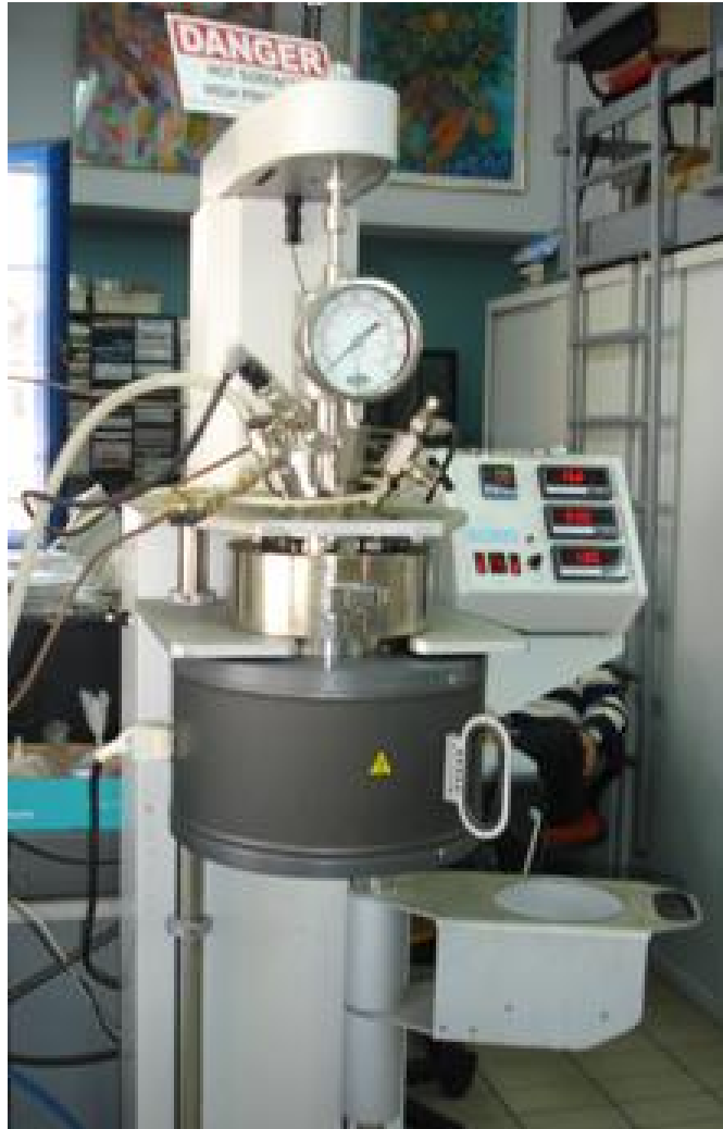
Fig .5.1 The 3.75-L batch reactor PARR 455
