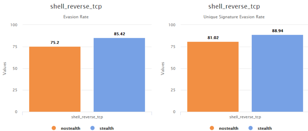
Figure 49. Evasion ratio and unique evasion ratio of stealth and no stealth mode for payload shell_reverse_tcp
