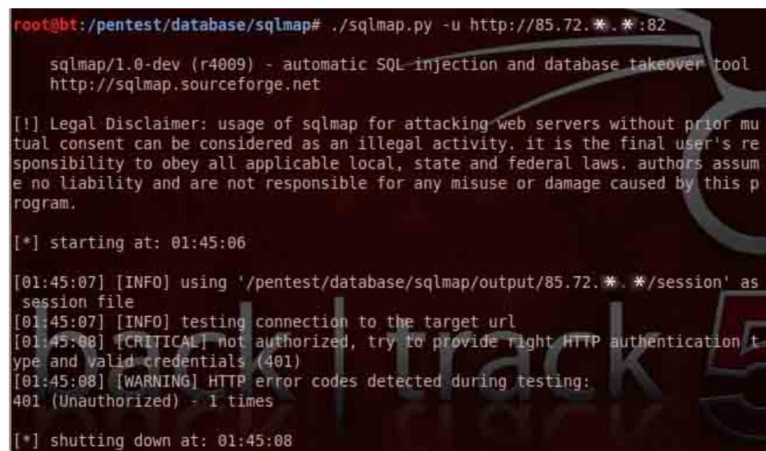
Figure 37: Automated SQL injection attack using Sqlmap
