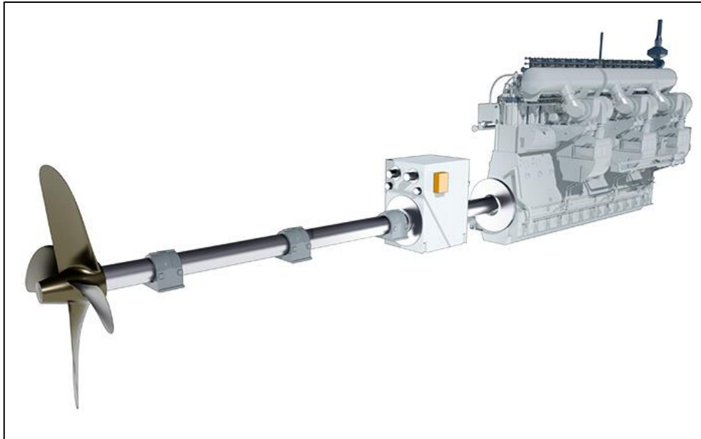
Figure 9: Shaft generator in concept design [42]
