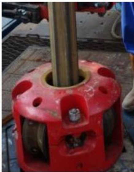
Figure 8 .Kelly fitted into drive bushing. (Autobahn Industries, 2023)
