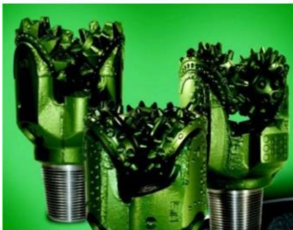
Figure 5. Tri-cone roller drilling bits ( K.Ngugi., 2008 ).
