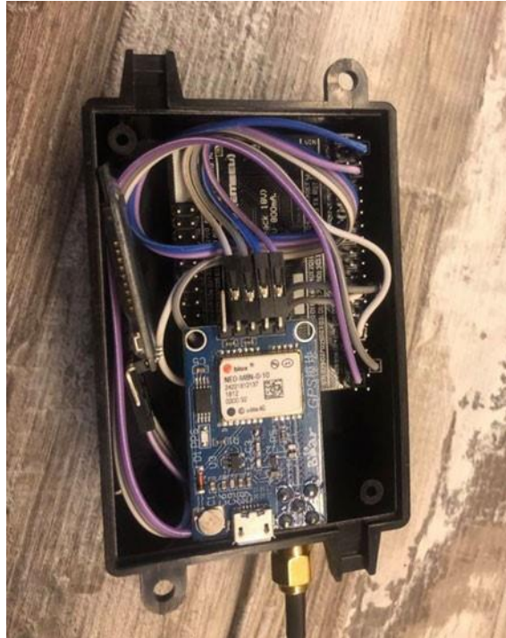
Figure 4.1. Blind RouteVision outdoor navigation—advanced field navigation sensor
