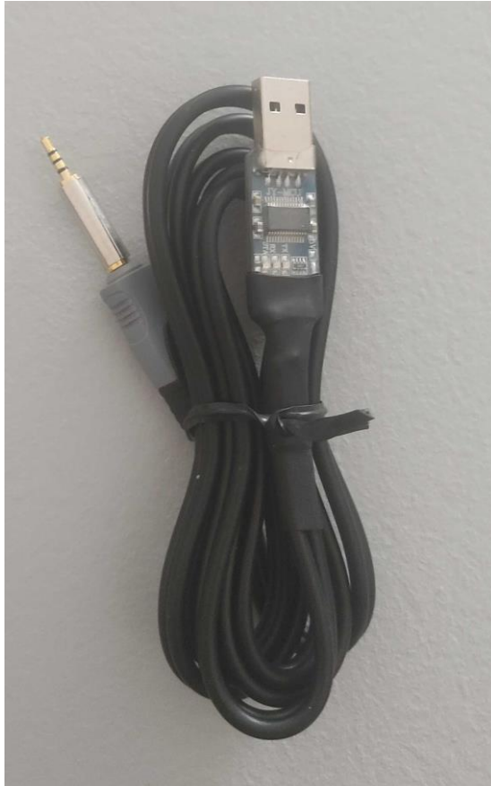
Figure 2.8 – Motorola T191 cable, including a CP2102 based USB-Serial converter.
