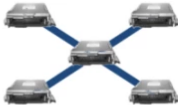
Image 10: FlexRay Star network configuration
