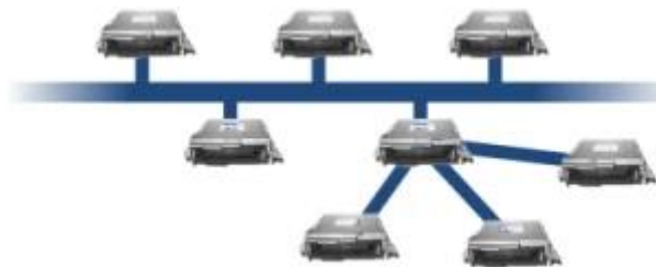
Image 11: FlexRay Hybrid network configuration
