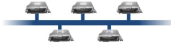
Image 9: FlexRay Multi-drop bus network configuration
