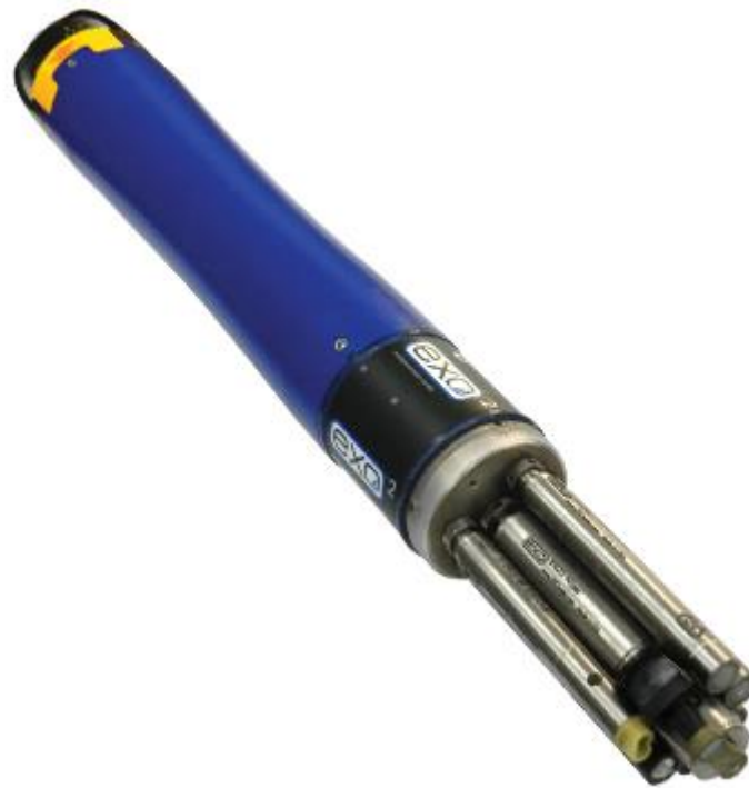
Figure 13. Multi-parameter Sonde (CTD) (sourc. Fondriest Site)
